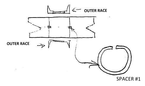
NOTE: These spacers set the preload of the tapered bearings by tying all the inner races together when the axle nut is drawn up.
