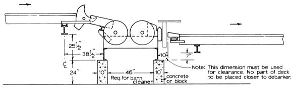
LIVE DECK with STOP & LOADER (std) STUB NOSE SKIDS DEBARKER 200 (36") & FOUNDATION OUTFEED DECK
