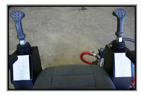
Armrest joysticks for ease of operation. Different brands and styles are available with custom button configurations.
