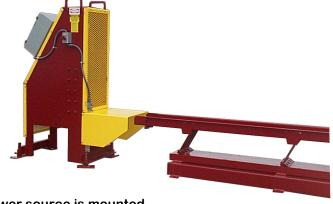
The hydraulic power source is mounted on a separate frame. The standard 20hp unit provides 10 cuts per minute while the optional 30hp unit provides 15 cuts per minute.
